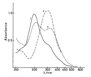
Figure 1. Absorption spectra of imidazolethione–iodine complexes in  $CH_2Cl_2$ : 1, [IT] 4.68 × 10<sup>-5</sup>M; 2, [1,3-Me\_2IT] 4.53 × 10<sup>-5</sup>M; 3, [1,4,5-Me\_3IT] 3.87 × 10<sup>-5</sup>M. Iodine concentration was in all cases 6.0 × 10<sup>-5</sup>M
