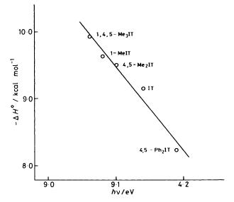
Figure 4. Plot of the frequency of the CT band maximum against the enthalpy of formation of imidazolethione-iodine complexes in methylene dichloride
