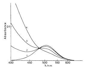
Figure 3. Effect of varying donor concentration on visible absorption spectra of imidazole-2-thione-iodine complex in  $CH_2Cl_2$ . [I<sub>2</sub>]  $6.0 \times 10^{-5}$ M. Concentration of IT: 1, 0.0; 2,  $2.34 \times 10^{-5}$ M; 3,  $4.68 \times 10^{-5}$ M; 4,  $9.36 \times 10^{-5}$ M
